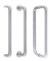
All window fittings, door handles, light fittings and hinges should be supplied in grade AISI 316 or AISI 444 in coastal areas, whilst grade AISI 304 is suitable for inland regions. To confirm this, request a letter from the supplier confirming the grade of stainless steel.
