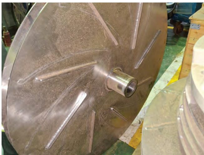
Impellers created from Sanicro® 35 plate. These have performed beyond expectation and have been corrosion resistant to high levels of sulphur.
