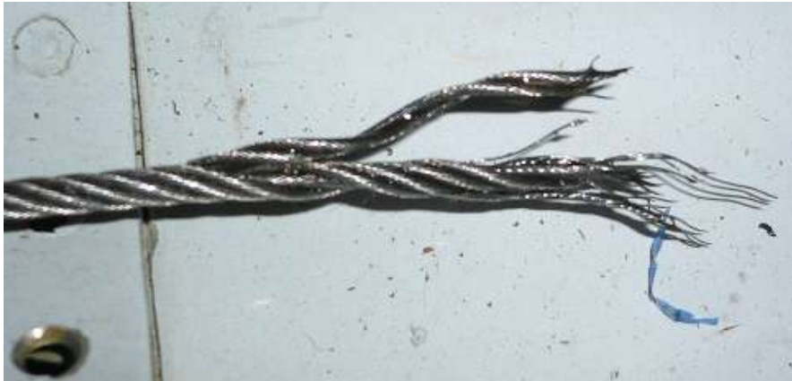
Aft failure of the pitch-up control cable (scale1:1)
